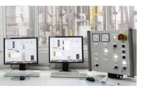
ALD provides precise control of all ESR remelting parameters for the reproducible production of homogenous ingots, which are free of macro-segregation and show a controlled solidification structure and superior cleanliness.
